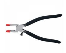
With adjustment screw and centre mark on upper jaw. Especially suitable for breaking narrow strips and glass thickness 3 - 5 mm Length 200 mm Jaw width 24 mm
