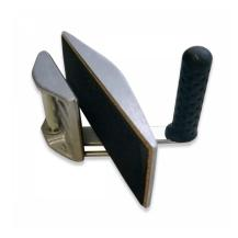
Heavy duty lifter that clamps to edge of sheet material such as glass, wood, steel, stone and much more. Max. capacity 80kg per pair. Designed for lifting by hand.
