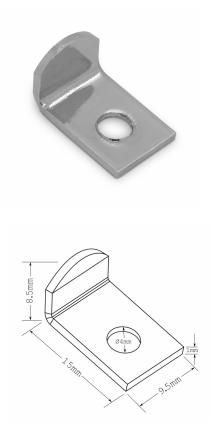
L shaped mirror clip for 6mm thick glass, with a 3mm countersunk fixing hole. Suitable for handling mirrors/frames etc.
