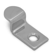
Z shaped mirror clip with a 12mm lip and 6mm return set for 6mm glass, with a 3mm countersunk fixing hole.
