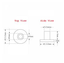
Rubber grommets to use as a buffer between the screw thread and the face of the mirror.
