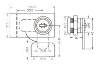
Cabinet swinging glass door lock for double door for glass thickness 5-7mm.
