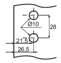
Available in both inset & overlay formats. Suitable for 5-8mm glass. 52 x 31 x 13mm. Max 12kg per pair.
