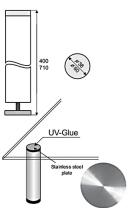
400mm high UV bonded table leg. Stainless steel mounting plate with polished chrome leg.
