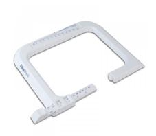
Glass thickness measuring device. Made from plastic, ideal for measuring the total thickness of pre installed insulated glass units. New extended type allows for the measurement around larger & deeper window and door profiles. A must have tool for anybody involved in unit replacement. The device is suitable for measuring glass thicknesses of up to 120 mm.
