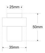
Made from Solid Stainless Steel SUS304 with black rubber.
