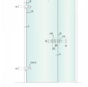
Ø12 - 14mm Ø12 -  $\bullet$  Prepared for both 8mm and 10mm glass thickness.
