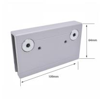
Suitable for use with the KODC730 overhead closer. For use with 10mm thick glass. No hole required in the glass. Used to mount the standard arm on a glass overpanel.
