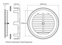
The Vent-A-Matic is a durable and effective in-glass ventilator that can solve most ventilation requirements. The PBS is equipped with an integral stormguard as standard, to reduce draft. Designed for use where continuous ventilation is mandatory. Marked with free air space to conform with gas board recommendations.
