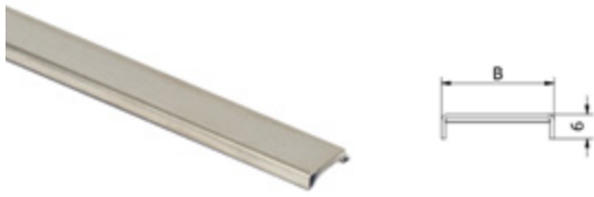
Edge protection, self-adhesive, AISI 316 brushed Edge Protection 6mm high and 1mm thick, sold individually.
