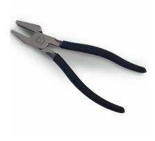
1"(25mm) jaw width, 8-1/2"(220mm) long, ideal for  $3{\sim}12mm$  thick glass. The flat upper jaw supports the top surface of the glass, while the lower hooked jaw enables glass to be cleanly opened at the cut line
