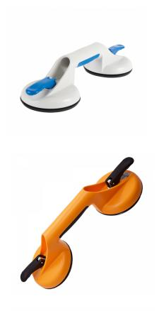
The Veribor® 2-cup suction lifter has a large, non-slip gripping area and lies perfectly in your hand. The levers have an ergonomic and user-friendly design. Their wide surface enables optimum force absorption. They are dimensionally stable but still soft enough to adapt to the surface during vacuum generation. The 2-cup suction lifter is suited for loads of up to 50 kg (two-fold safety factor) and can be used for all materials and objects with gastight surfaces.
