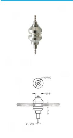
11mm hole, 5mm to 8mm glass. WEIGHT LIMITATIONS: When properly installed, loading weight for 4 wires (one range) is 38kgs, loading weight for each shelf is 12kgs.
