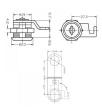
Cabinet swing glass door lock for double doors for glass thickness 5-6mm. Accessories:
