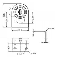
Cabinet swinging glass door lock -19mm cylinder - zinc alloy. • Comes with 2 Key Alike keys
