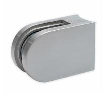
A 63mm x 45mm D shaped 304 grade polished stainless steel clamp. Suitable for mounting on a 48/50mm diameter post. Used mainly indoors for stairs, glass balconies, counter dividers, retail glass displays and splash guards. Supplied with an OPTIONAL anti slip safety pin which allows you to drill the glass to ensure that it never slips downwards over time. These clamps are suitable for loads up to aproximately 34kgs per four clamps.
