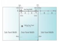
A = [Over Panel Width - (180 + 180)]÷2 B = [Side Panel Width - (180 + 180)]÷2 Complete G-Tech single door kit with glass mounts. Suitable for a single glass door mounted on two glass side panels and an overpanel. Maximum door weight: 100kg.
