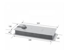
Closing Ranges: Two closing speed variable by valve adjustment provide full hydraulic control Valve 1: 130-20 degrees closing speed. Valve 2: 20-0 degrees latching range.
