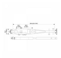
Type "S" Side load arm assembly. For top rail with 12.5mm recess.  $\,$
