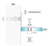
It consists of turned articles and screws in stainless stell AISI 316L to fix the angle bracket between glass and wall.
