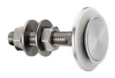
Fixed bolt with a countersunk head for use in spider glazing systems. Manufactured using 316 grade stainless steel. Standard 65mm long axis and suitable for 15 - 22mm thick glass. Please see the other bolts in the range for additional glass thicknesses. Special dimension glass bolts available on request. Glassparts recommend using thread locking compound whenever possible. These items are not held in stock and will require
