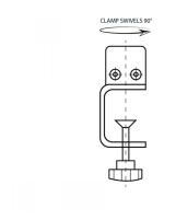
• Our Stainless steel desk partition clamp can be used with glass, acrylic, polycarbonate, wood, metal etc.
