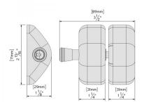
Gate Magnetic Latch is made from 316 marine-grade stainless steel. It adapts to many mounting applications. Blind fixed from the rear optimises the sleek finish with no visible fasteners.
